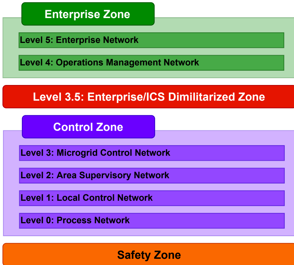
Figure 2-1. Microgrid Network Logical Architecture
