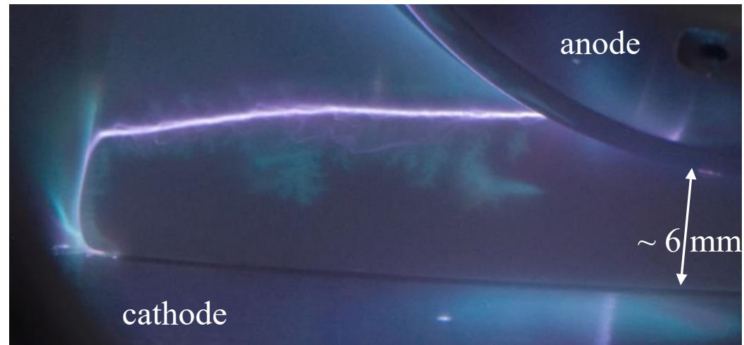
Time integrated image of lateral surface flashover with branching primarily reaching towards the cathode. ( \sim 240 kV)
