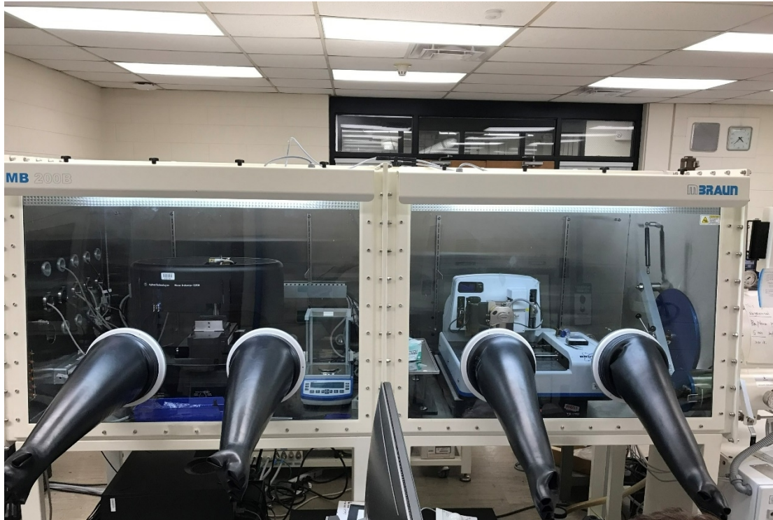
Left: G200 Nanoindenter and Bruker Dimension Icon AFM in glovebox
