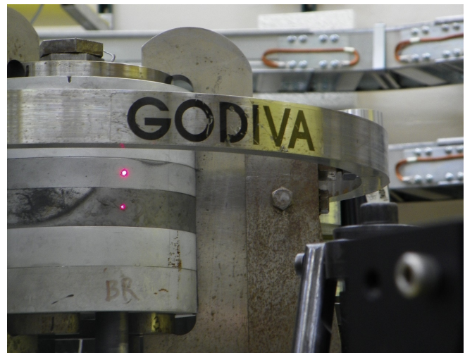
Figure 1: Visible Laser Indicating Target Positions on Godiva IV Core
