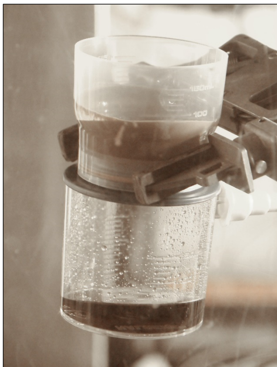
Figure 3-17. SME Product during vacuum filtration
