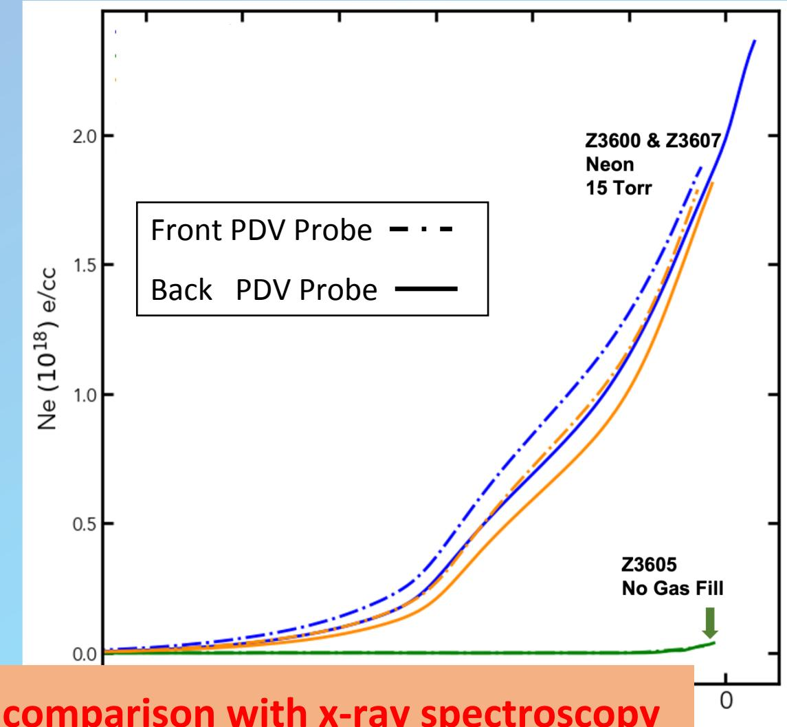
Electron density measurements allow comparison with x-ray spectroscopy measurements as well as comparison with simulation
