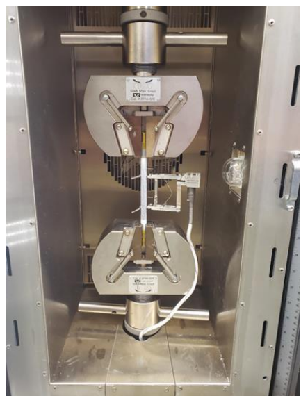
Axial tube tensile test
