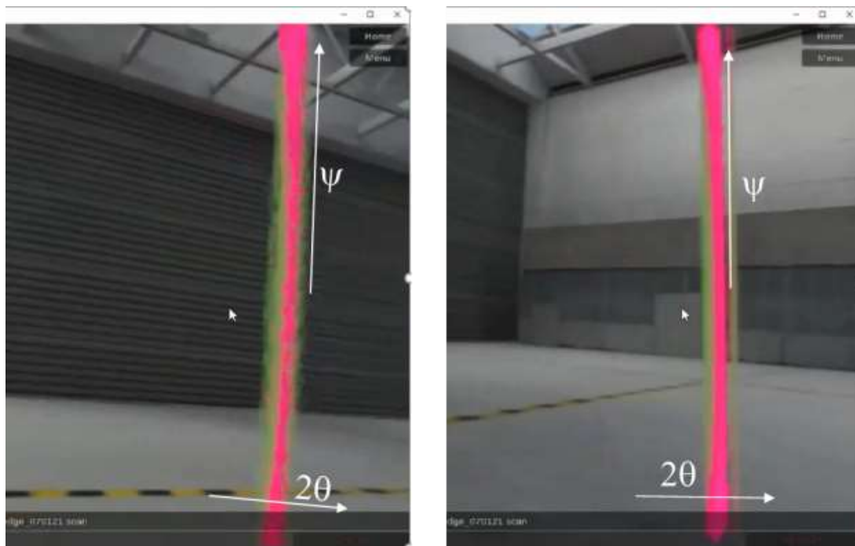
Figure 11. Reoriented view of cross-sectioned pole figures for \alpha -W (211); low counts (green) and high counts (magenta). Left: raw data showing possible warp in intensity along \psi direction. Right: pole figure cross-section of extracted Factor 1 dataset with reduced noise and clearer detection of concave warp toward lower 2\theta indicating presence of in-plane tensile strain.
