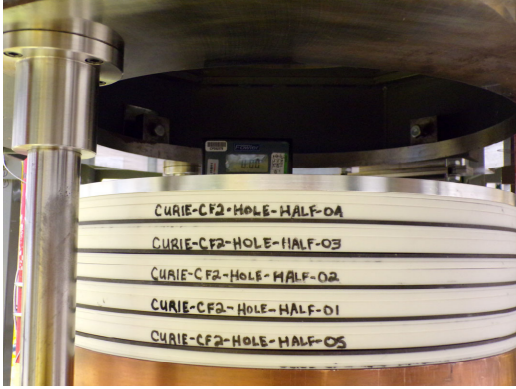
Fig. 2. Bottom portion of the core loaded with 7/8" Teflon
