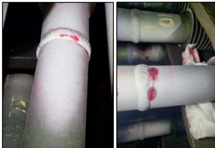
Figure 2: Images showing the locations and appearance of the tube leak sites at the tube-to-tube welds after PWHT and hydrostatic testing.
