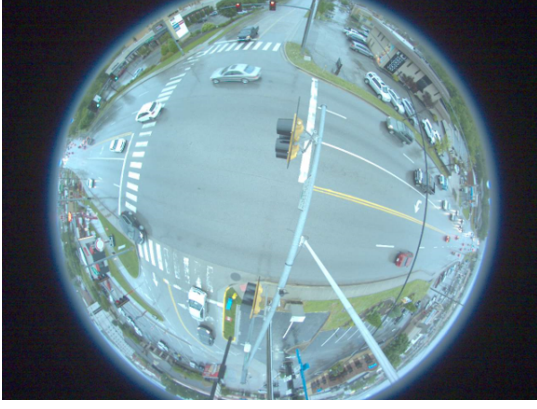
Fig. 1. The fisheye view of a GRIDSMART camera. The sensor detects vehicles as they arrive at the intersection. It estimates each vehicle's speed and it tracks vehicles as they move through the intersection to determine their turn directions.
