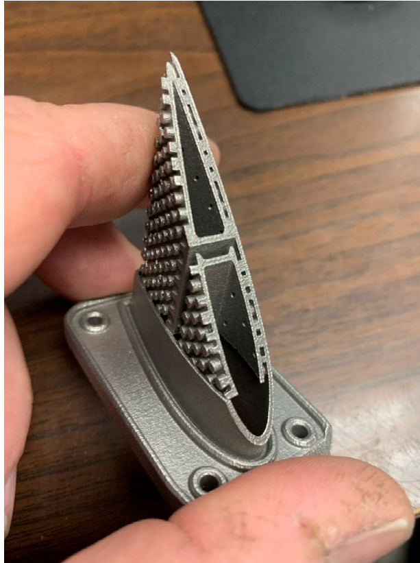
Figure 22: Partial AM print of the incremental impingement geometry showing base, pedestals, cold-side impingement holes, and central plenum.
