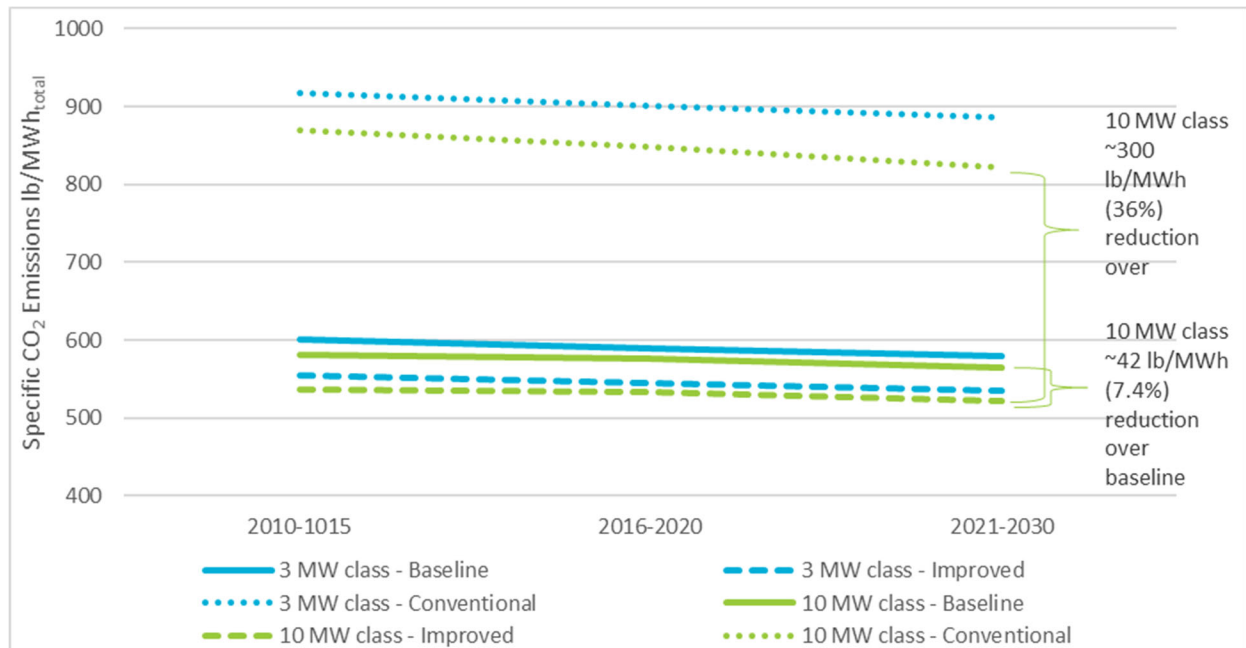
Figure 5: 3 MW and 10 MW specific CO 2 emissions based on total (electric and thermal) output. Adapted from Theis et al. (2020).
