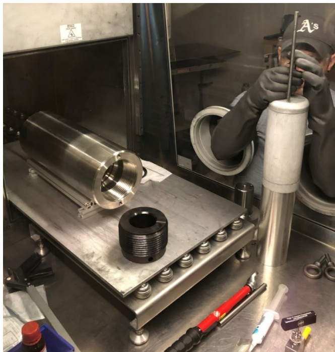
Figure 4-31. Prepping the inner subassembly to be inserted into the pressure vessel.
