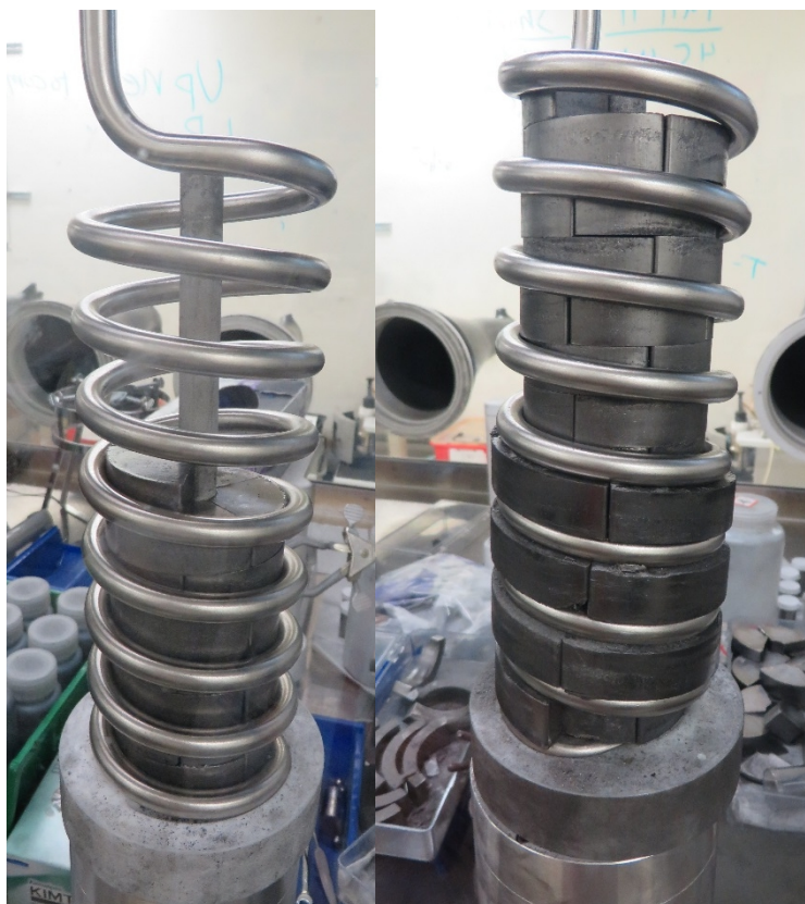
Figure 4-30. Helical coil being filled with center pellets (left) and then helix pellets (right).
