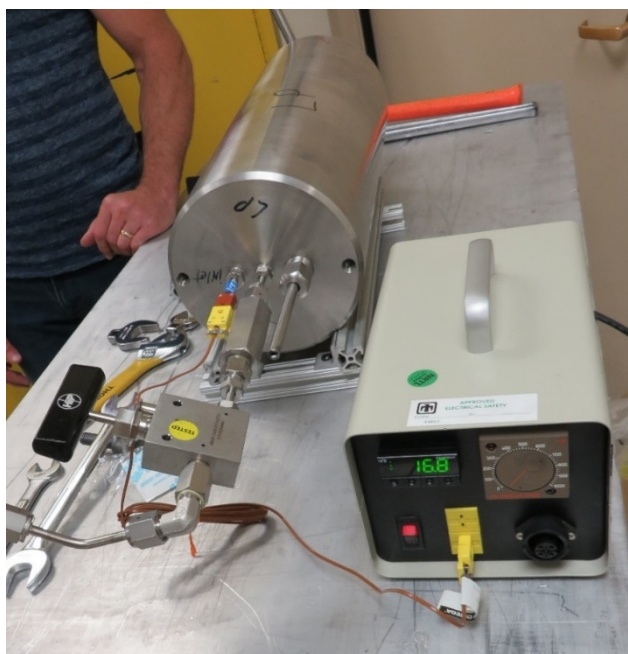
Figure 4-32. LP bed during He leak check and thermocouple verification.
