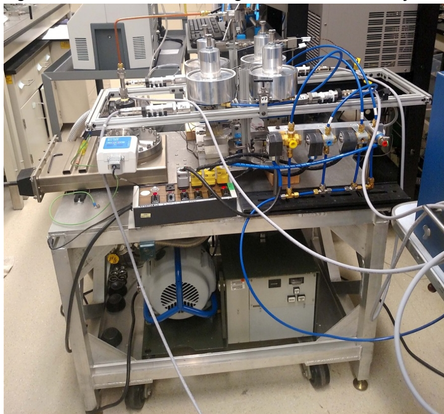
Figure 2-3. Schematic of initial design of the ORNL Sieverts system.
