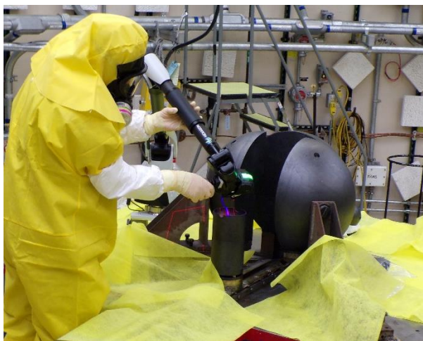
Fig. 2. CMM scan measurement of Flattop pedestal.
