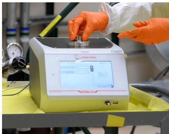
Fig. 5. Loading sample in small cell into pycnometer.
