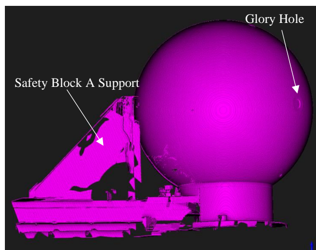
Fig. 4. Digital rendering of CMM scan for closed Flattop configuration showing support for safety block A and glory hole.
