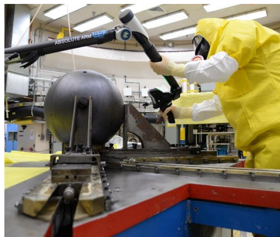
Fig. 3. CMM scan of Flattop while closed with HEU core removed.
