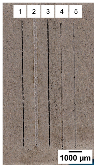
Figure 3.1. Top-down macro image of the five melt tracks completed on the C103 sample. Each melt track is labelled 1-5 which corresponds to parameters detailed in Table 3.2.
