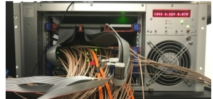
4 CAEN V1742 32-channel, 5 GSs -1 , 12-bit digitizers (DRS-4 chip)
