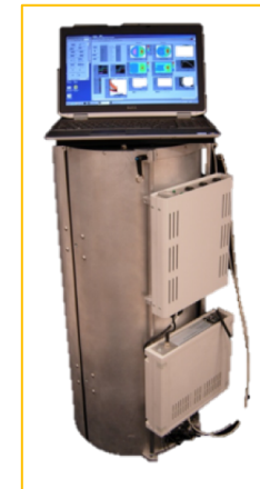
Mobile Imager of Neutrons for Emergency Responders (MINER)
