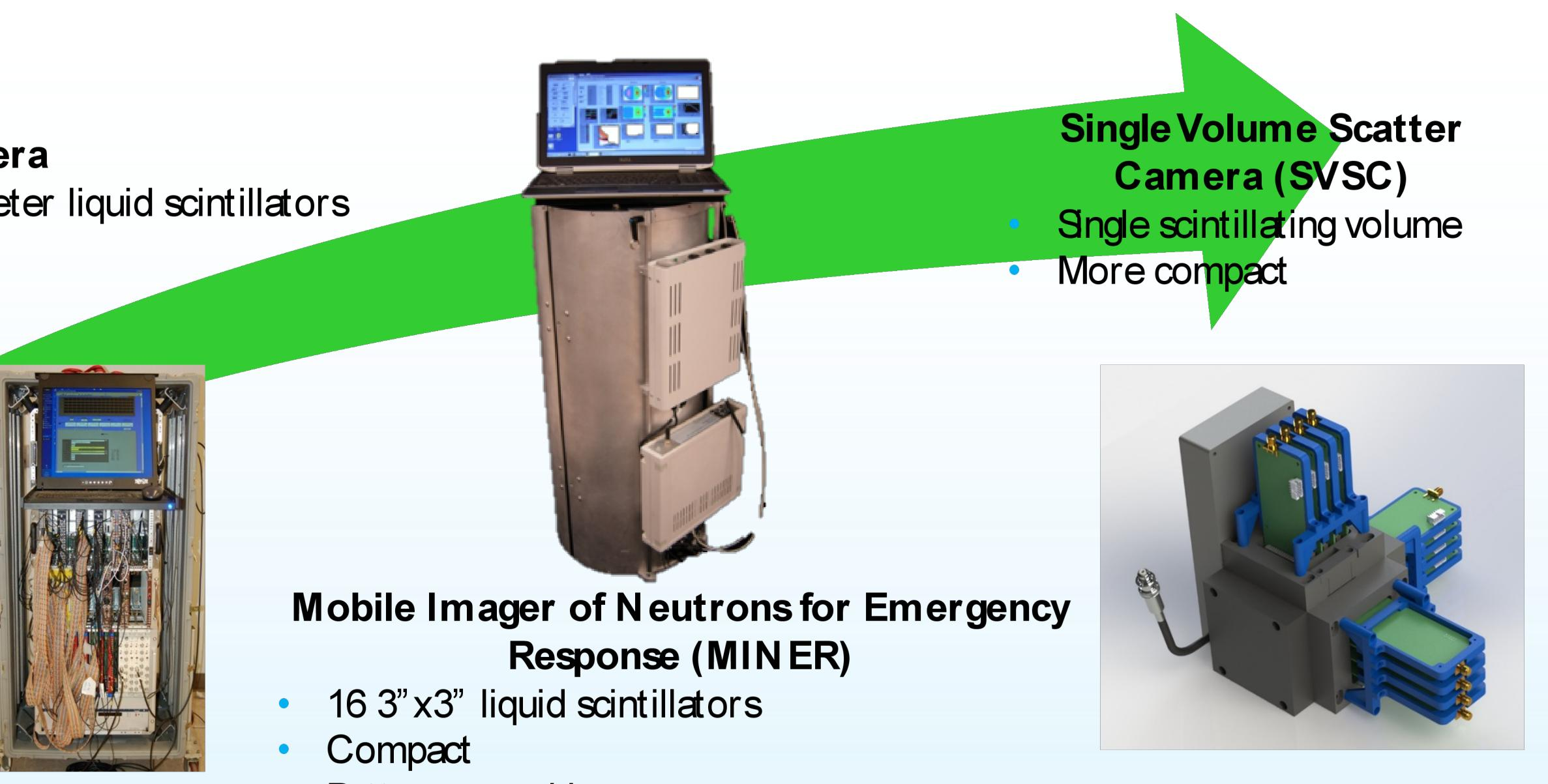
R&D on neutron emission detection has been an evolution towards compact and portable technologies that are easy to transport and deploy, have high efficiency, and can be placed near an item to increase sensitivity & spatial resolution.
