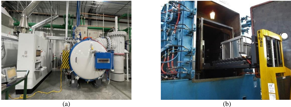
Figure 3. (a) Vector high-pressure gas quench furnace type 20VP-669 at the Seco/Vacuum facility and (b) the Phoenix™ HTS12 system assembled and loaded into the Wellman vacuum oil-quench furnace.
