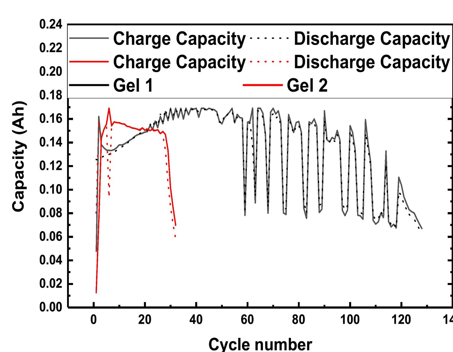
Industrial prismatic cells were fabricated with PAA-KOH gel for the 2<sup>nd</sup> electron technology. This application is under development to perform longer cycle life
