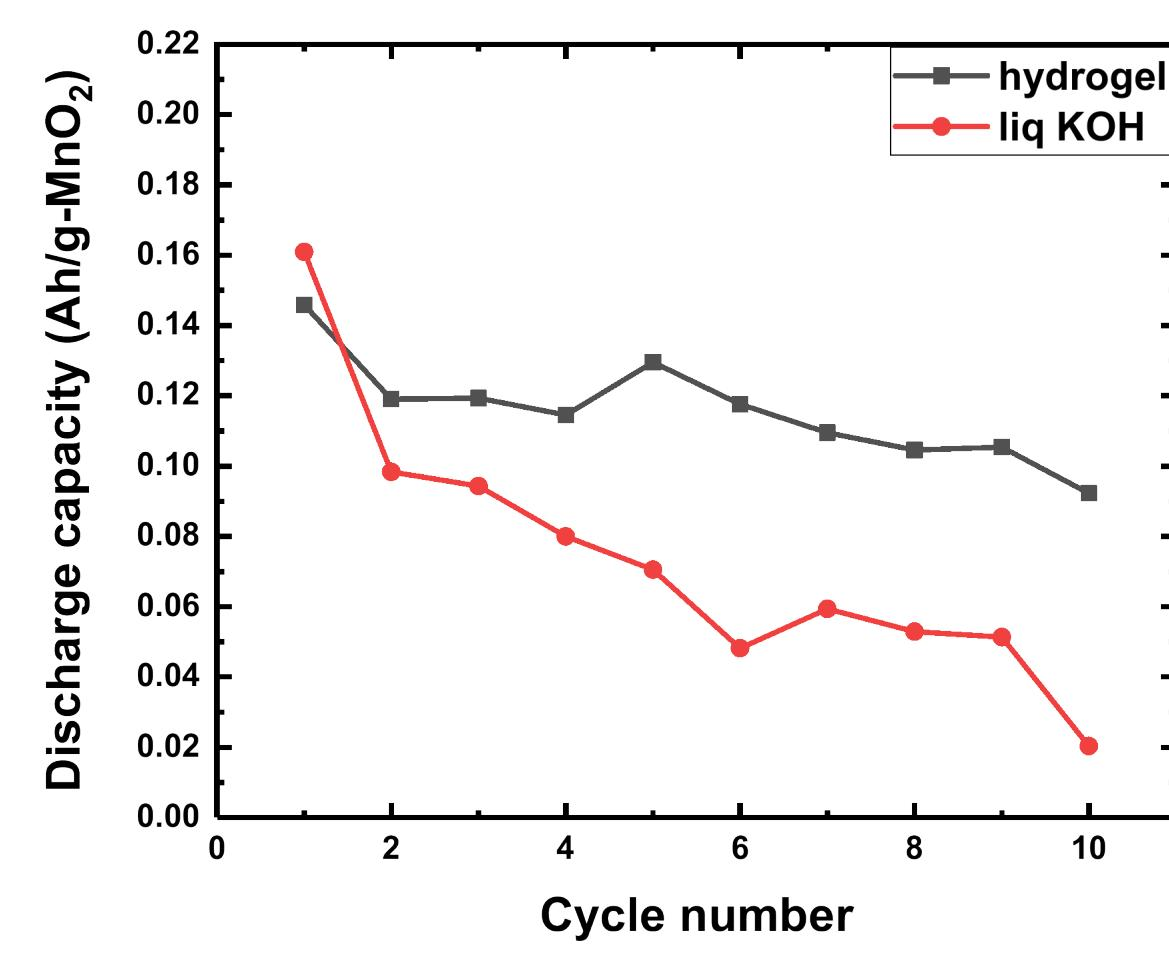
Discharge capacity during cyclic voltage scans across the 1<sup>st</sup> electron reaction window is improved by used of PAA-KOH hydrogel electrolyte
