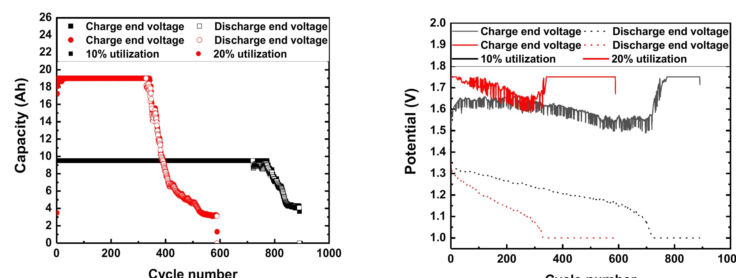
Industrial prismatic cells of were fabricated with PAA-KOH gel and other cells with traditional liquid KOH electrolyte. PAA-KOH gel electrolyte cells survive greatly more cycles than cells made with the liquid KOH electrolyte.
