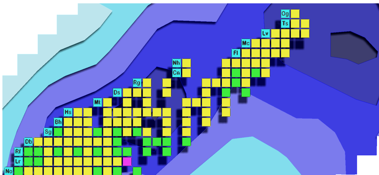
Figure 1.1: Nuclear Chart with the Island of Stability. Known isotopes are shown by their preferred decay mode, either alpha (yellow), beta (magenta) or spontaneous fission (green). These are on a backdrop of predicted shell effects from [Sob01].
