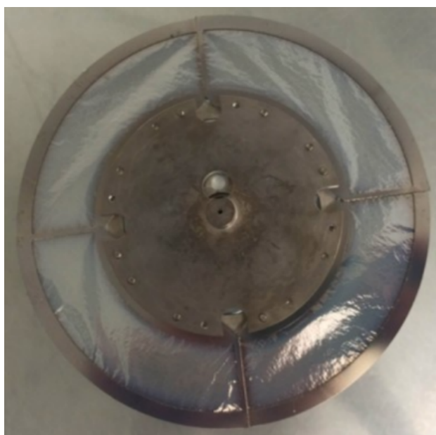
Figure 6.1: ^{209}\text{Bi} target produced via vapor deposition
