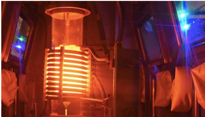
Figure 4: Images of casting operations inside glovebox.
