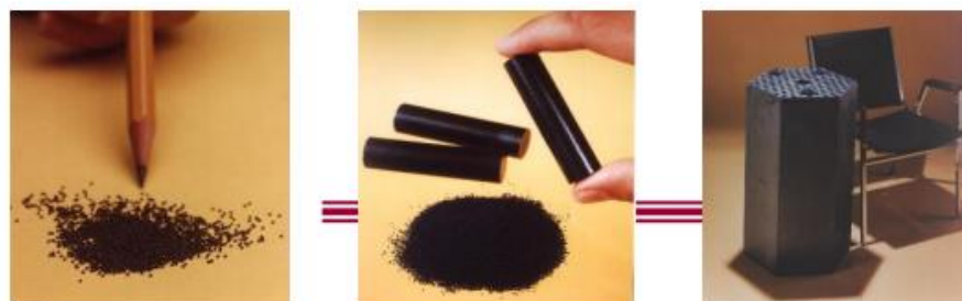
Figure 8. TRISO fuel kernels (Left), cylindrical fuel compacts (Center), fuel element blocks that will hold fuel compacts (Right) (General Atomics, n.d.)
