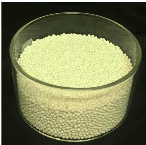
Figure 19. Round 1 CO 2 sorbent produced by Porocel.
