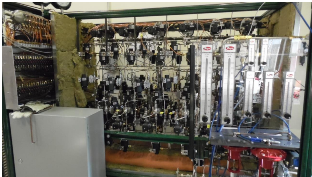
Figure 22. TDA Bench-scale apparatus with 10 beds for continuous adsorption and regeneration
