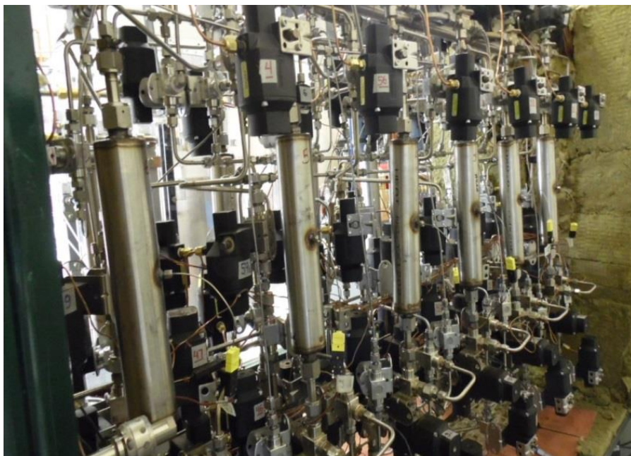
Figure 7. CO 2 Capture bench-scale (5L sorbent) apparatus with 12 bed (Two rows of 6 beds with one row of beds shown in front).
