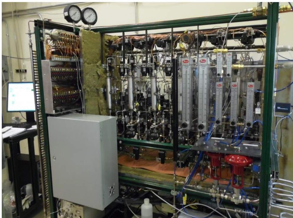
Figure 6. TDA Multiple fixed bed bench-scale apparatus
