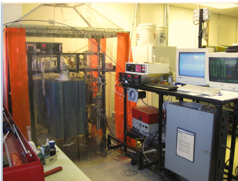
Figure 20. TDA single fixed bed sorbent testing apparatus
