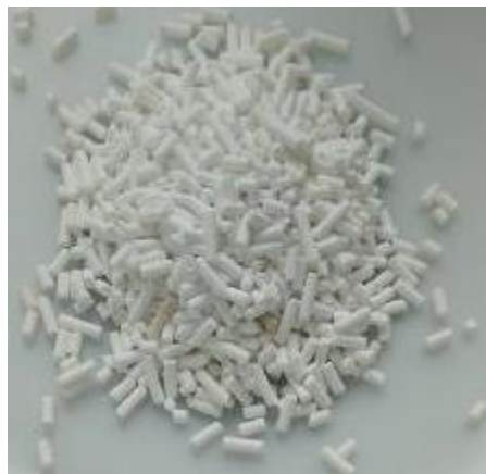
Figure 23. Round two customized extruded sorbent prepared by Porocel
