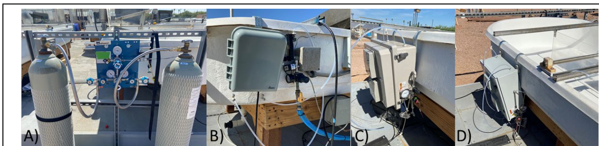
Figure 5.2. A) Gas regulator installation next to raceways. B) Installation of mass flow meter box on a sparging raceway. C) Mass flow meter and gas analyzer box on raceway 1. D) Primary data logger box and mass flow meter and gas analyzers on raceway 2. Note that raceway 3 has an identical box to that on raceway 1.
