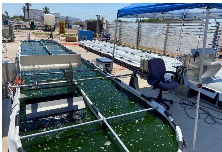
Figure 8.1. Installation and setup of 25-m 2 raceways on the westside of the AzCATI field site at ASU. Note that raceways were designed and built by the staff and students of AzCATI.
