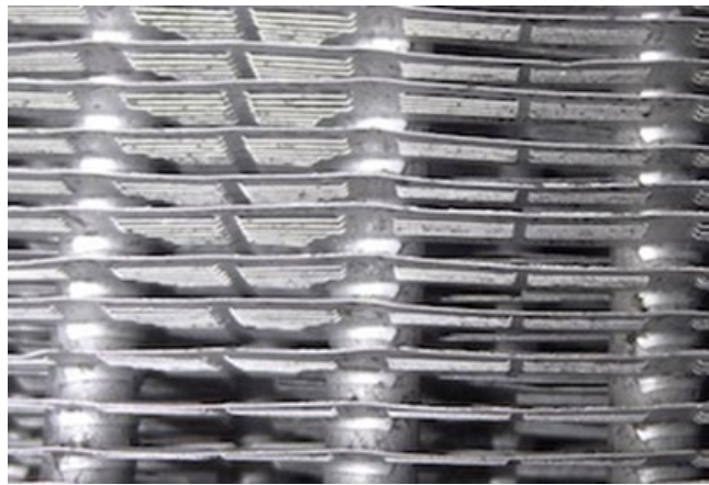
Figure 98: SubZero Prototype, Brazed Fins to Tubes
