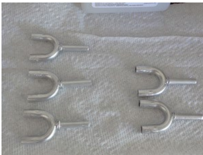
Parts assembled before flux and braze
