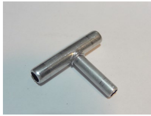
5.55mm tube into the 7mm clad tube + braze ring
