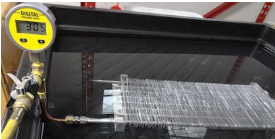
Figure 99: SubZero Prototype Leak Pressure Test
