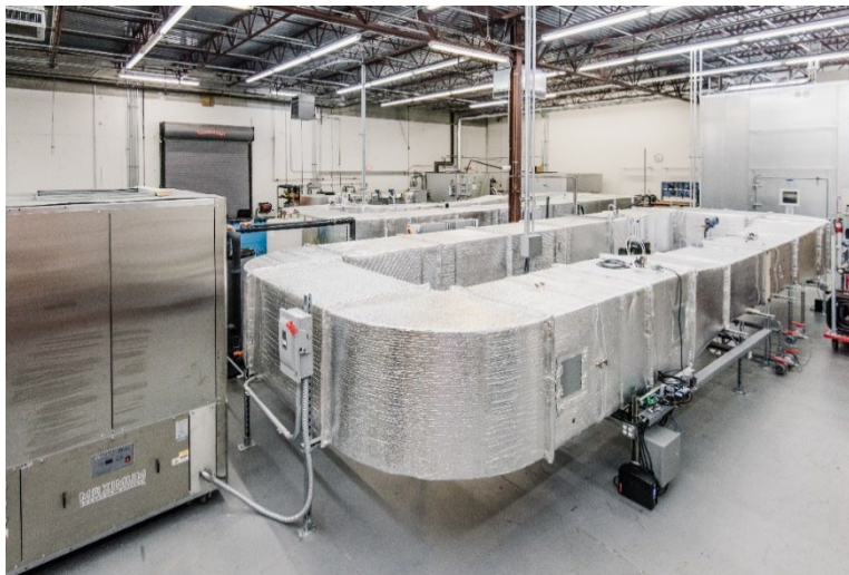
Figure 75. View of OTS laboratory, including temperature and humidity-controlled wind tunnels.
