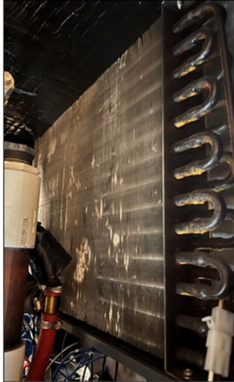
Figure 94: Baseline Carbone Steel Heat Exchanger in the SMTI Heat Pump Water Heater
