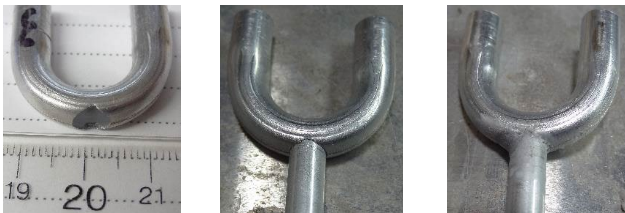
Figure 58. Split-Merge brazed connections
