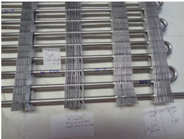
Figure 88: Testing of Fin Material and Proposed Collar Adjustments
