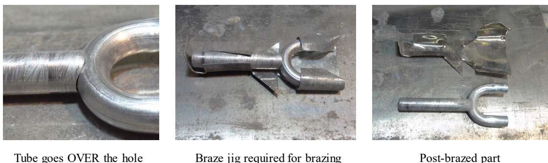
Figure 59: Initial Braze Tests.
