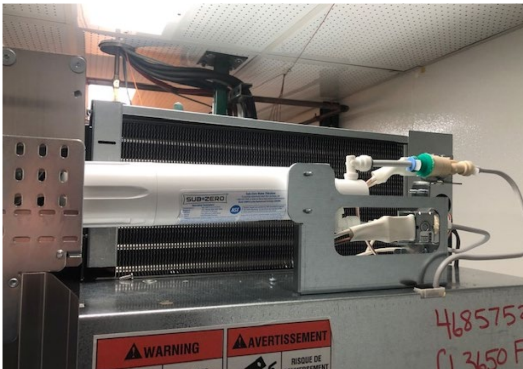
Figure 101: Tube-Fin Baseline Heat Exchanger in Sub-Zero System Assembly
