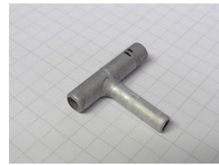
Brazed part, no jig required
