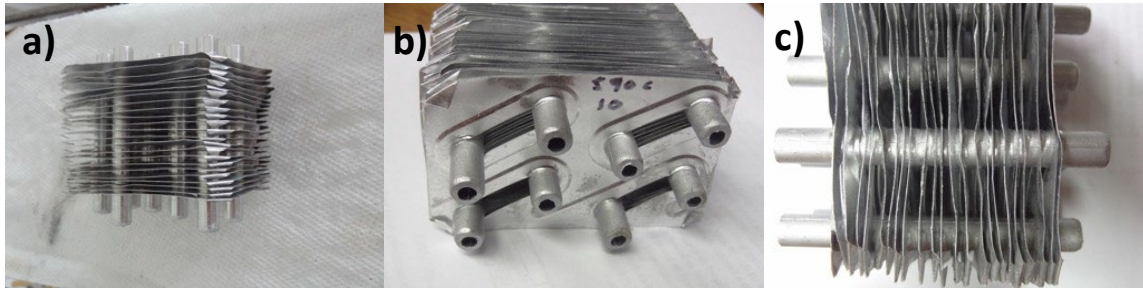
Figure 50: Result of Test 8: a) Sample with 8 tube-24 fins prior; b) Good braze joints; c) Good braze joints across
