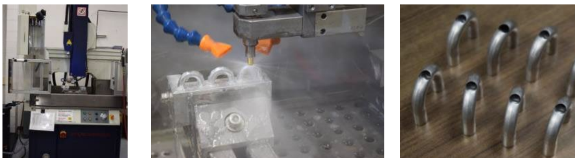
Figure 57: Split-Merge holes using EDM
