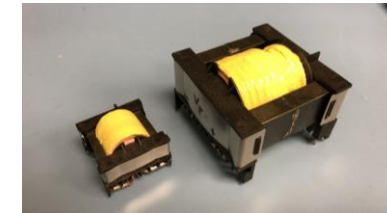
High-frequency transformers for current prototype (60W) and forthcoming converter revision (600W)
