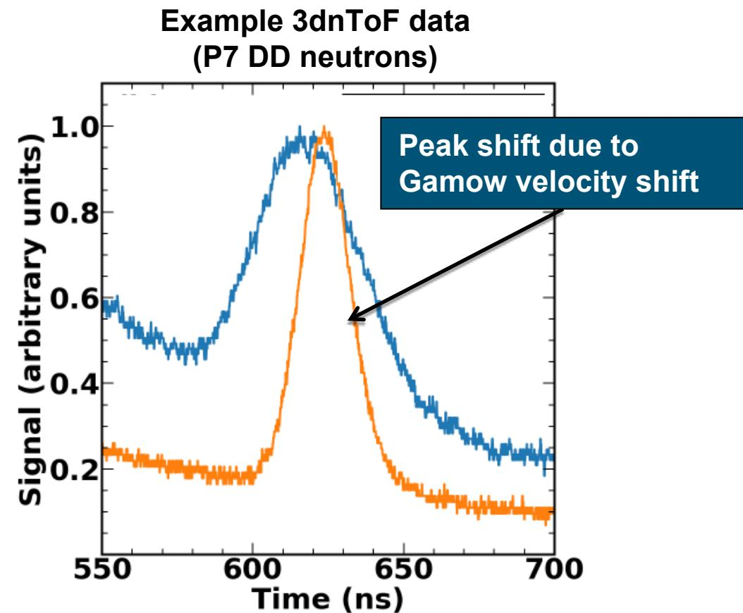
The plasma apparent ion temperature, bulk velocity, and Gamow shift was inferred from these measurements
