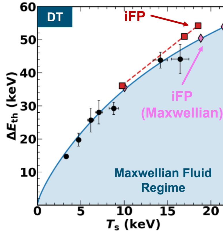
The iFP bimodal ion velocity distribution predictions are consistent with the high temperature DD measurements
