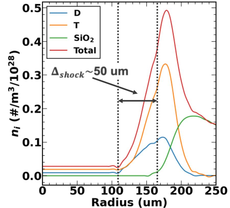
The long mean free paths leads to a smoothing out of the implosions shock front
