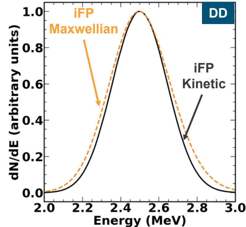
The bimodal ion velocity distribution produces a narrower neutron energy spectrum
