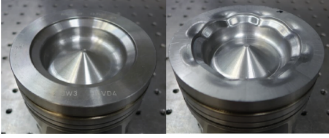
Figure 7. SL and DSL pistons used in engine experiments. The DSL piston has been machined in-house from a piston blank.
