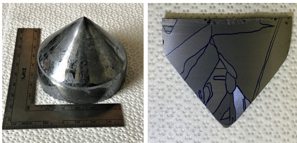
Figure 19: CG-245 ingot and wafer slice
