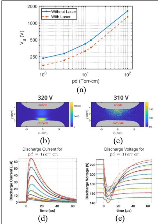
Fig. 1 – (a) Breakdown voltage versus pressure times distance ( $pd$ ) in argon with and without laser-induced photomeission. (b) and (c) show images of laser-induced breakdown at 10 Torr-cm and the transition to Townsend discharge at 315 V. (d) and (e) show that, for 1 Torr-cm, the laser-induced discharge current and voltage (solid lines) can match a 0D model at low currents/space charge (dotted lines).
