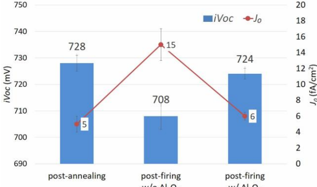
Fig. 3. Measured iV_{oc} and J_0 from the samples with and without Al 2 O 3 capping layer after simulated high temperature firing process
