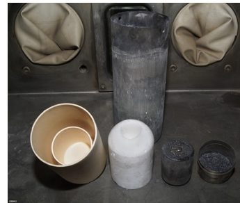
ER setup (left to right): Crucible, salt, feed metal, \text{PuCl}_3
