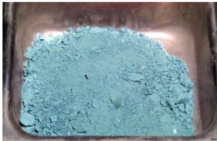
Metal chlorination salt containing 3-5% Am and remainder Pu
