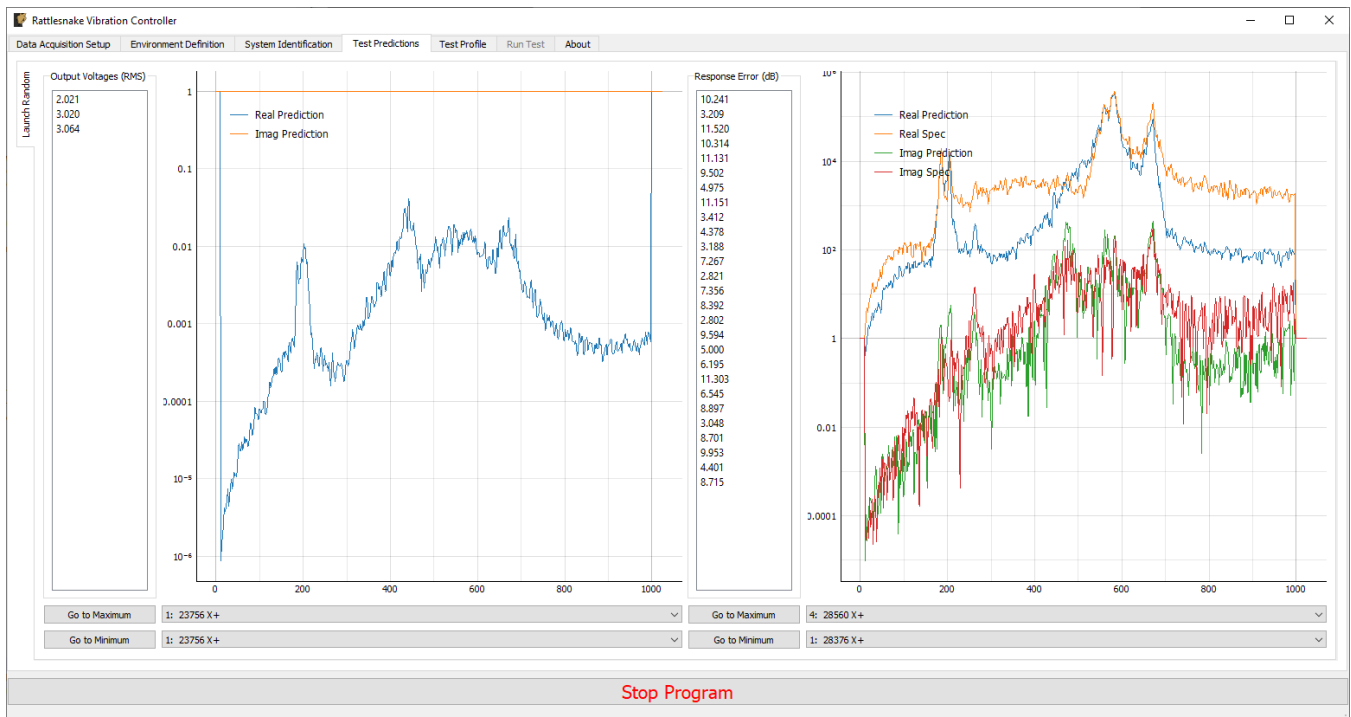
Figure 6: Visualizing the test predictions on the Test Predictions tab of the Rattlesnake controller
