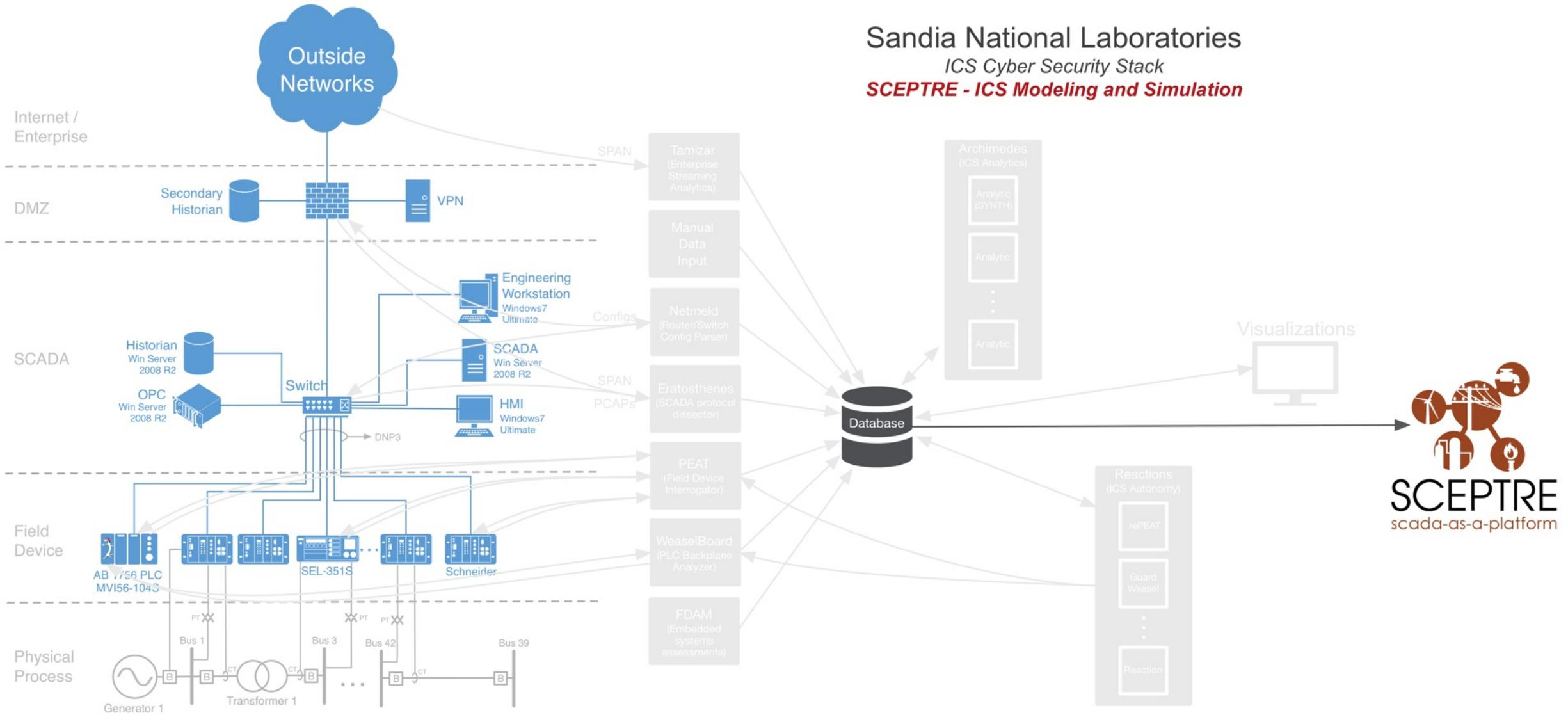
*SCEPTRE provides a comprehensive ICS/SCADA modeling and simulation capability that captures the cyber/physical impacts of targeted cyber events on critical infrastructure and control systems*
