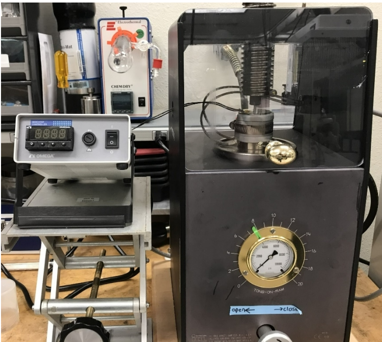
Lab scale hot pressing set up
