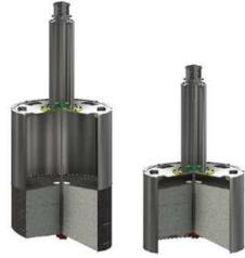
Core retention in core bit. Left: start of cut. Right: end of cut.
