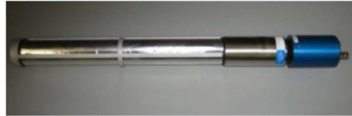
*Direct-Push Prototype Beta Detection Probe*
