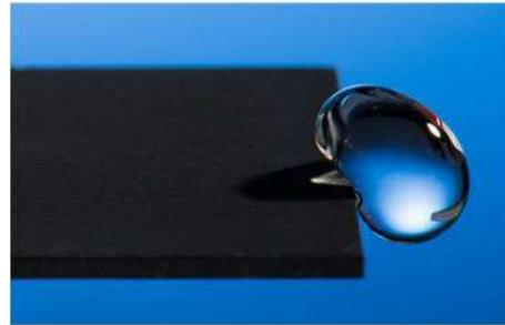
*Water repelled by laser treated surface*
