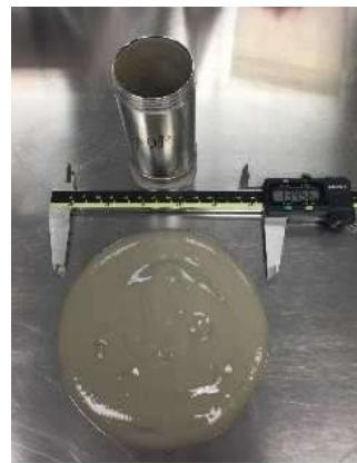
*Grout Flow Testing of Encapsulation Grout*
