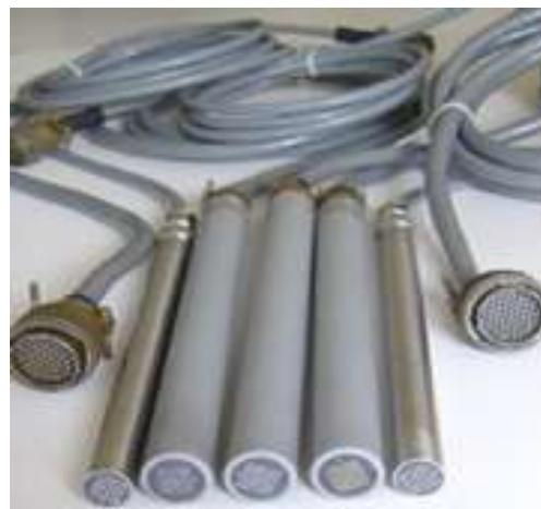
*NanoCorr Tank Corrosion Probe*
