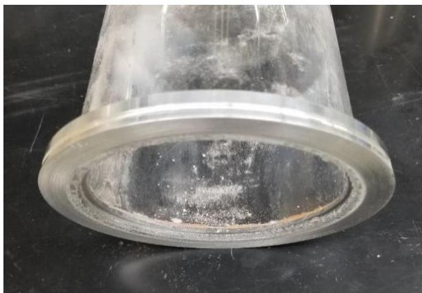
Figure 1.1-12. Corrosion of the Al bottom flange after exposure for 2 h to Ar that had been passed over non-purified \text{MgCl}_2\text{-KCl} -bearing salt for 2 h at 750°C
