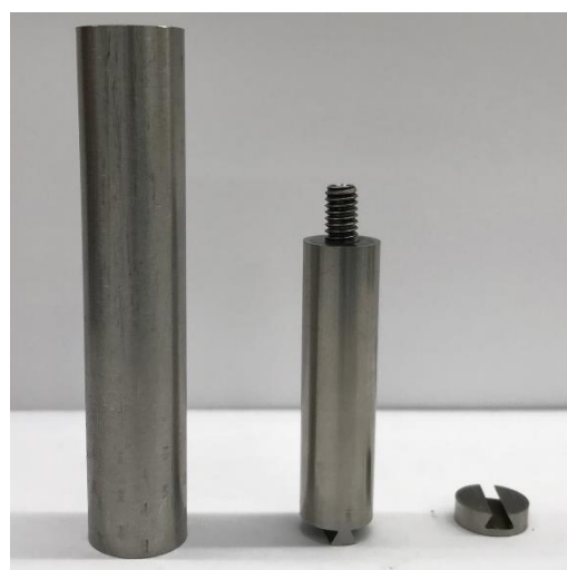
Figure 1.1-6. Photograph of a 316 SS outer sleeve (left), a 316 SS sample holder (with dovetail extension, middle), and a 316 SS sample (with dovetail groove, right)
