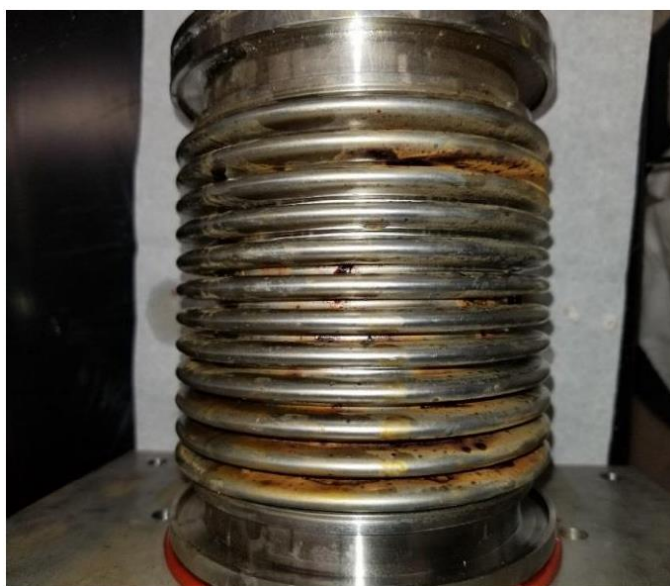
Figure 1.1-11. Excessive corrosion of the bottom stainless steel bellows, after exposure for 12 h to Ar gas passed over non-purified \text{MgCl}_2\text{-KCl} -bearing salt at 750°C
