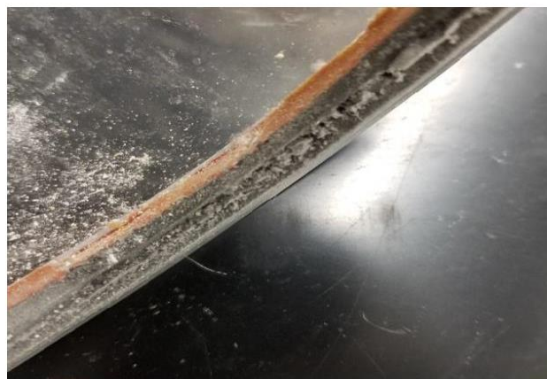
Figure 1.1-12. Corrosion of the Al bottom flange after exposure for 2 h to Ar that had been passed over non-purified \text{MgCl}_2\text{-KCl} -bearing salt for 2 h at 750°C
