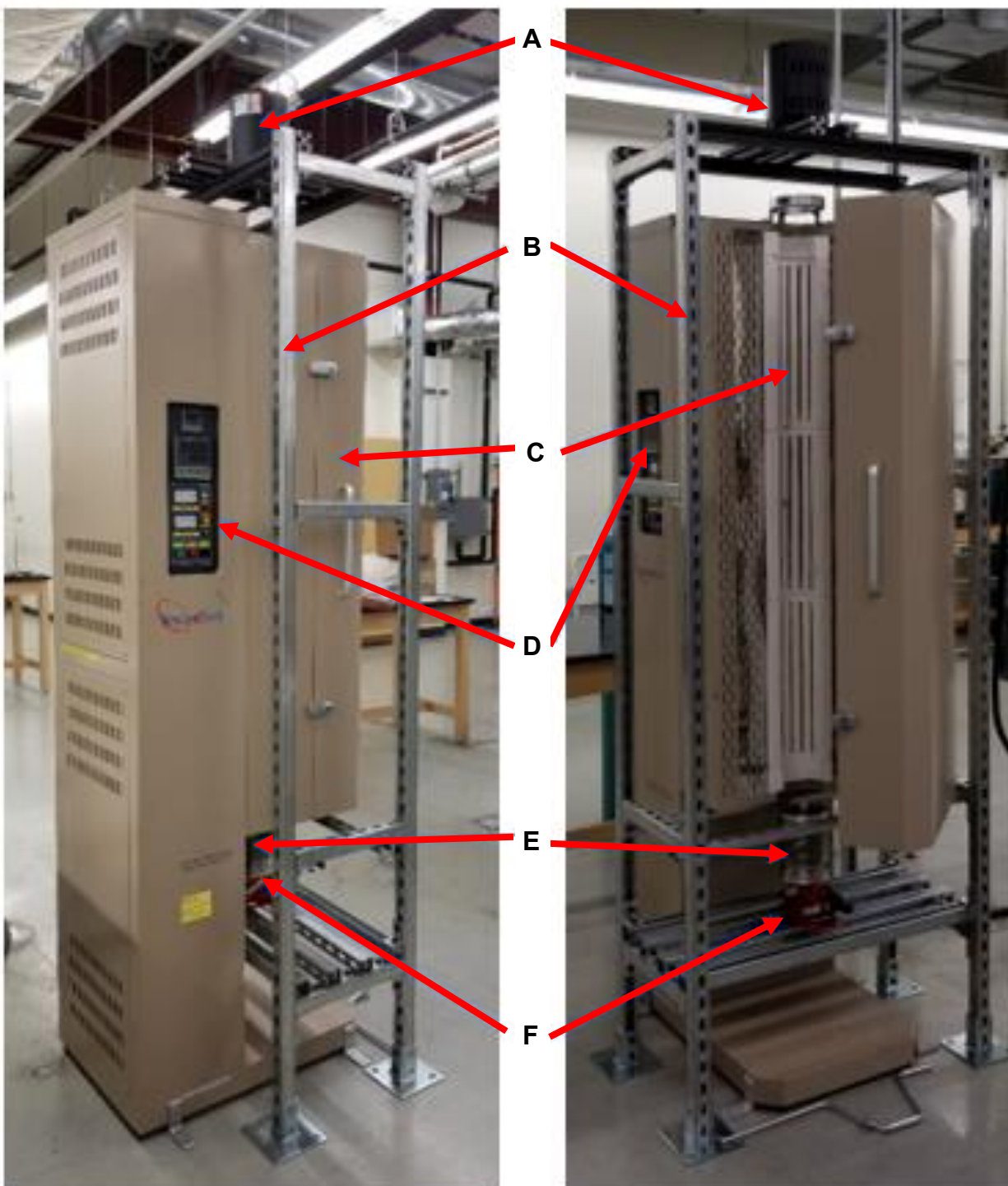
Figure 1.1-2. Photographs of the rotating-disk apparatus revealing components: A = motor, B = steel support frame, C = clamshell vertical (electrically-heated) tube furnace, D = furnace controller, E = compressible bellows, and F = scissor lift jack
