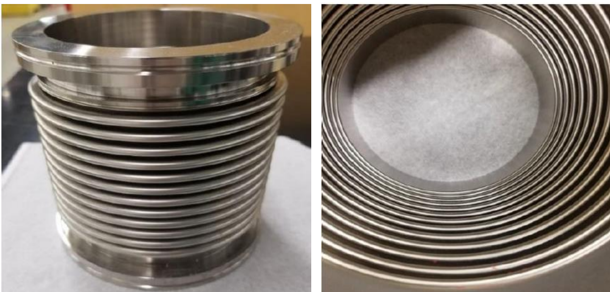
Figure 1.1-14. Photographs of the inspected bottom bellows after exposure to Ar gas passed over \text{MgCl}_2 -KCl-bearing salt at 750^\circ\text{C} for 6 h
