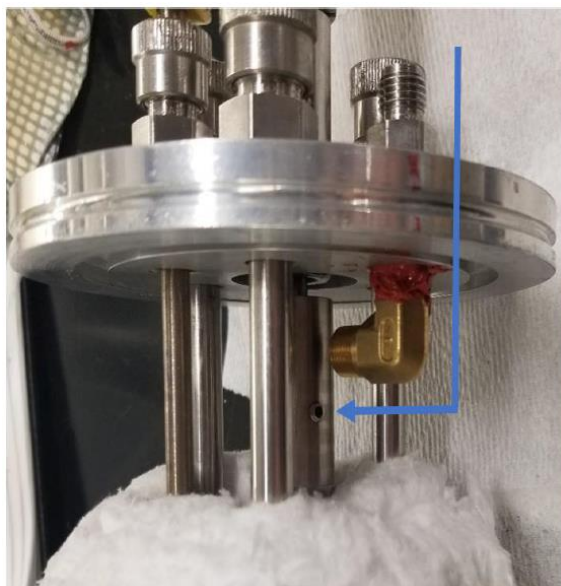
Figure 1.1-10. Photograph of the modified top assembly, with the blue arrow depicting redirection of inlet gas flow for active cooling
