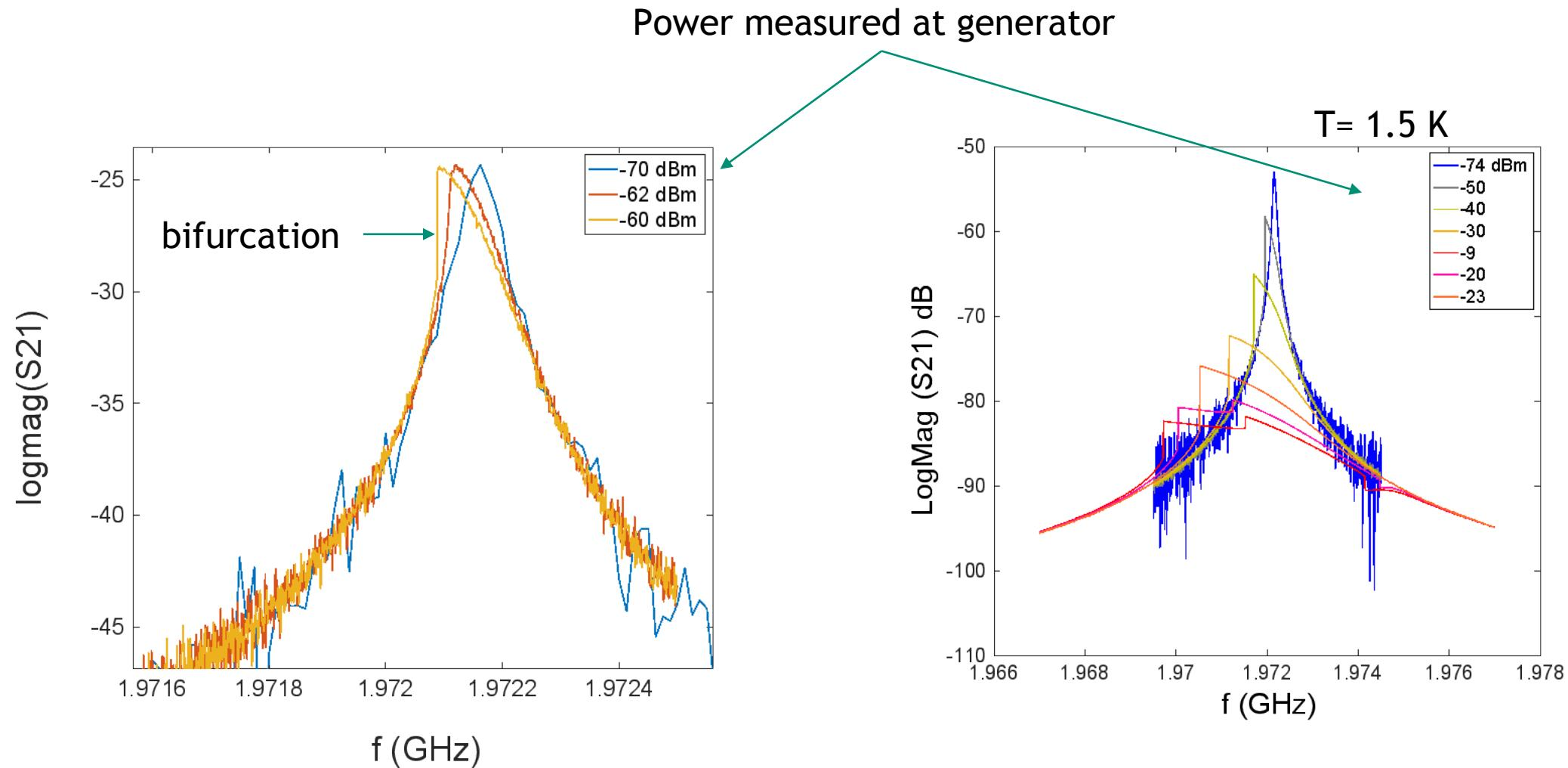
Peaks translate to lower frequency due to increased kinetic inductance ( $L_k$ ) as power increases
