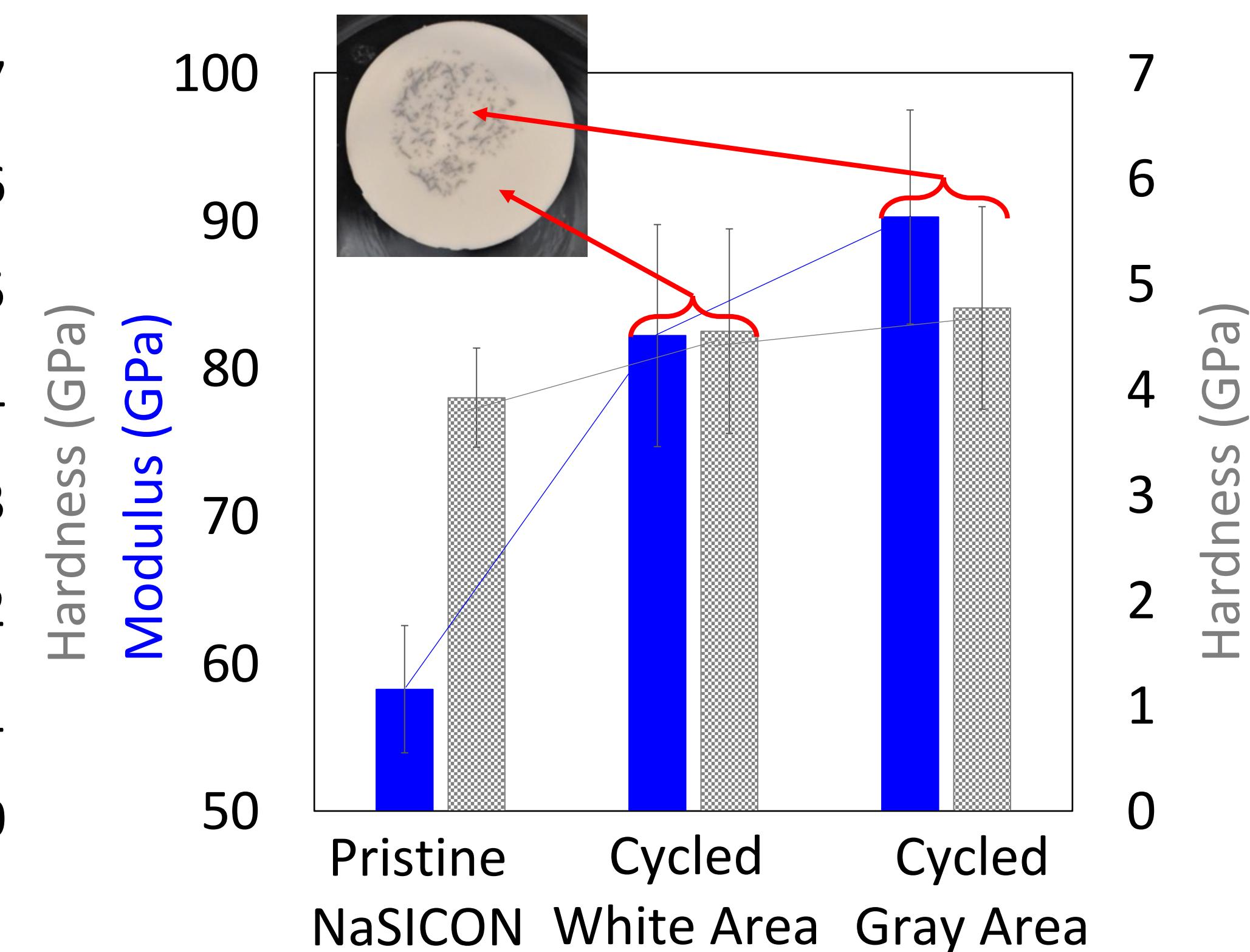
Excessive cycling can precipitate new phases that increase modulus and hardness
