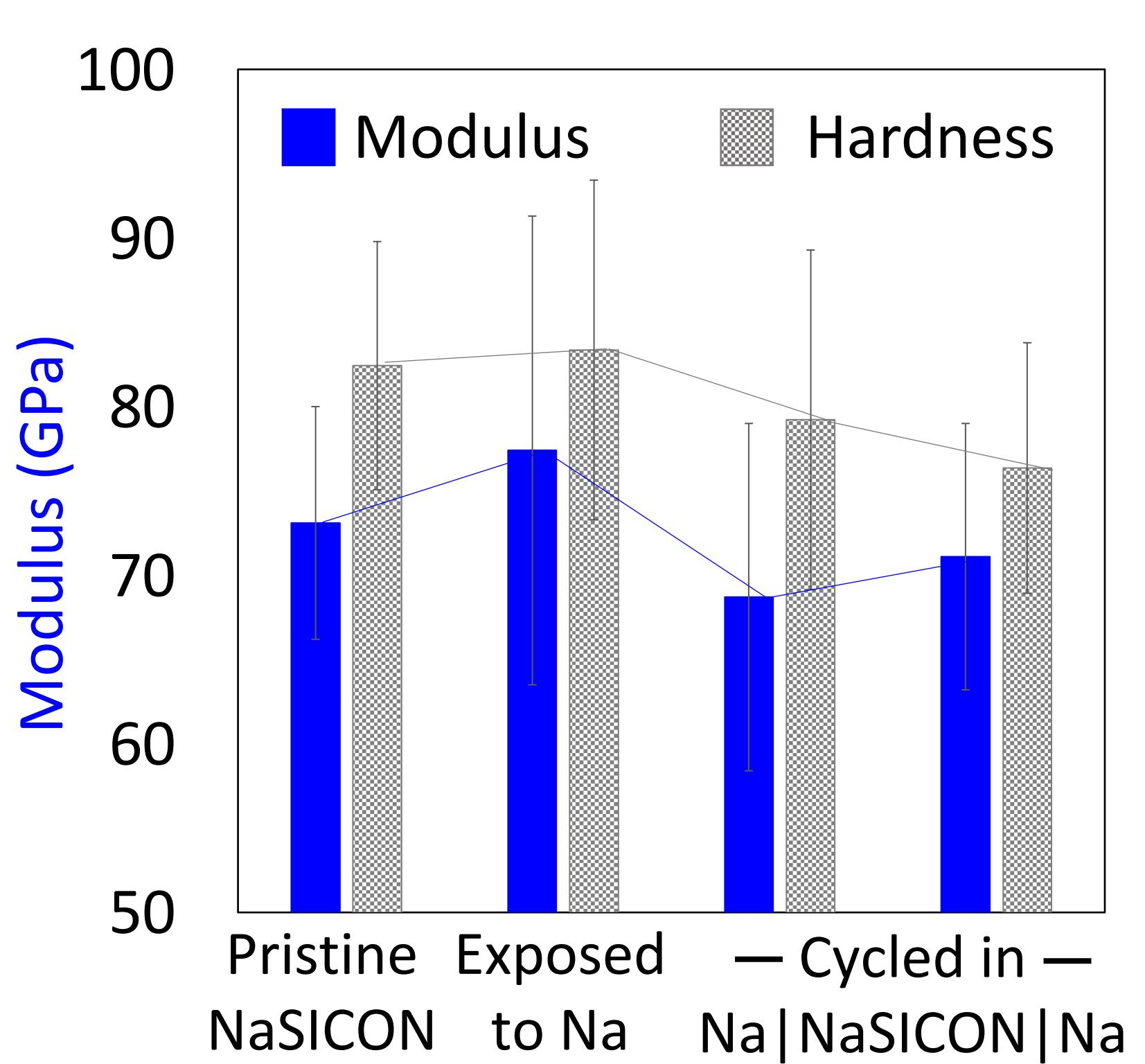
Sodium conduction causes mechanical changes in NaSICON.
