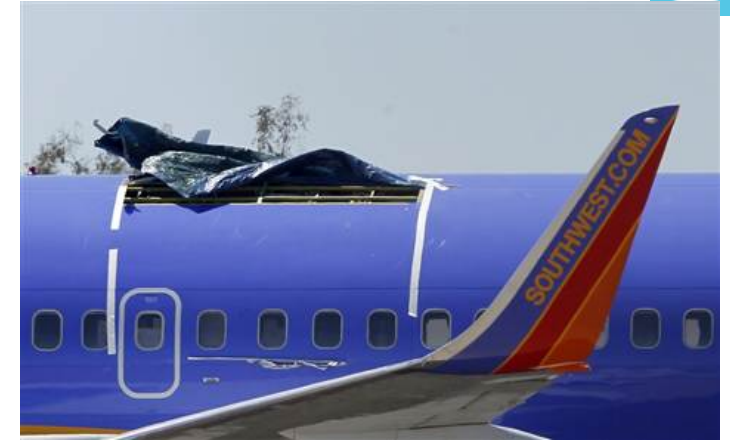
Above: roof failure of Boeing 737 aircraft due to fatigue cracks. From imechanica.org
