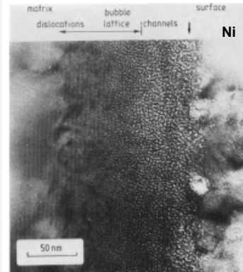
FIGURE 8. Transverse section of a high dose He-irradiated surface layer of Ni showing inter-connected channels, bubble lattice and dislocations (TEM micrograph by Jäger, 2002).
