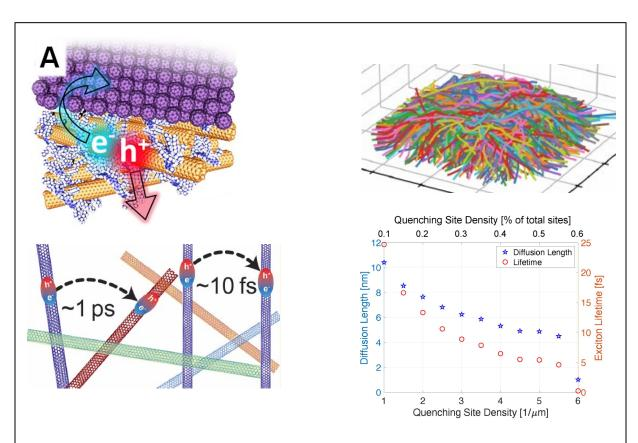
(**Top left**) Schematic of exciton dissociation a thte interface between a carbon nanotube film and a C60 layer. (**Top right**) Numerically generated carbon nanotubes film. (**Bottom left**) Shecmatic of exciton transfer between nanotubes and characteristic rates (fast between similar parallel tubes, slow between different misoriented tubes. (**Bottom right**) Calculation of diffusion length in DECaNT.
