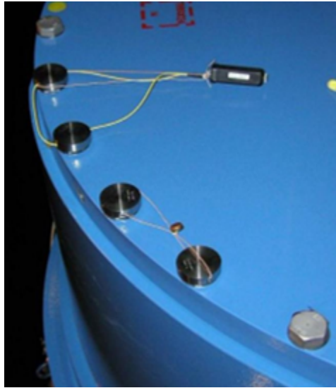
Figure 3: Casks are sealed with two different seal types. Electronic seal is shown on top, and metal cup seal is shown connecting two bolts on the bottom of the image. Image from [8].
