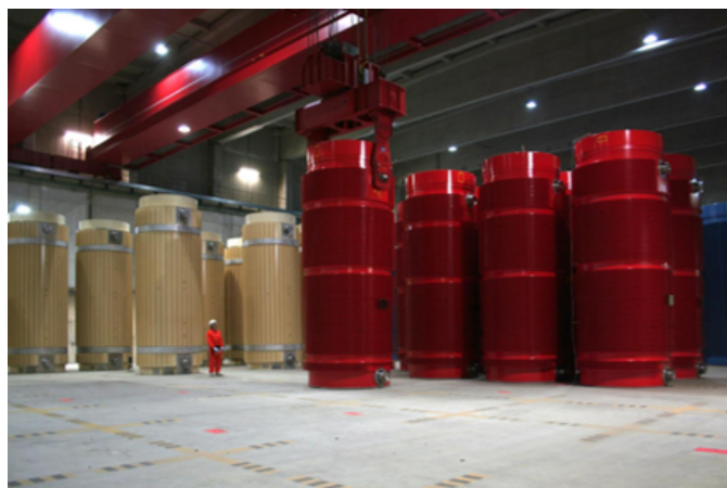
Figure 4: Casks can be large, with access to the seal only from the top. Image from [8].
