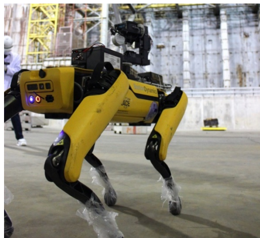
Figure 10: Spot, with a radiation detection payload, deployed at Chornobyl. Image from [15].
