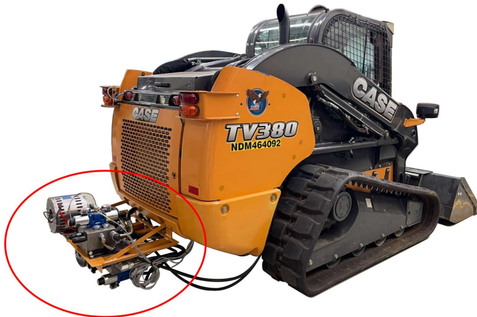
Figure 45: Demonstration on the reference vehicle, with two EHA systems to drive the boom and bucket functions
