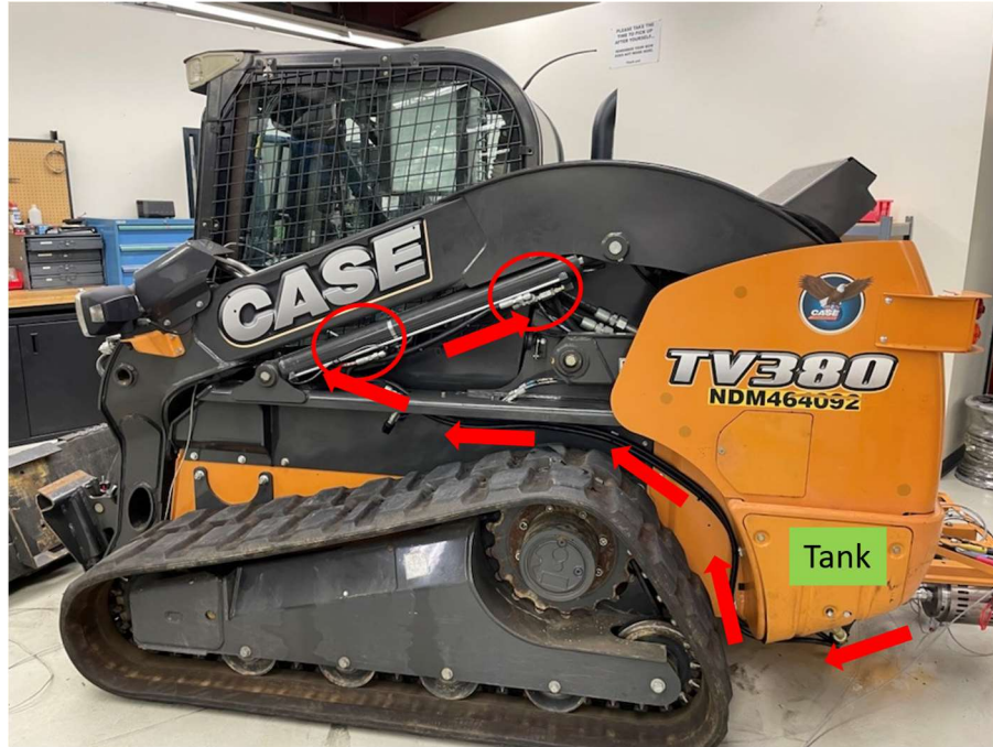
Figure 46: Hydraulic configuration on the reference machine
