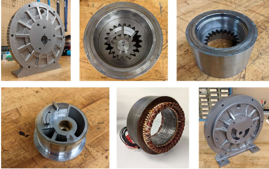
Figure 60: Top row, from left to right: EHU end-lid; EM rotor, pinion and radial compensation system; EM rotor with highlight of the metal sleeve protecting the magnets. Bottom row, from left to right: bottom HM casing with axial compensation system; EM stator; bottom end-lid.
