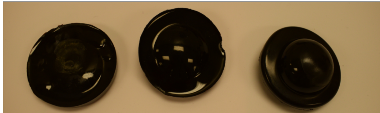
60 Co Gamma Irradiated – Dose Rate = 641.4 rads/s - 190 hours
