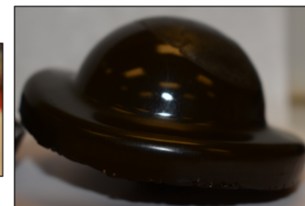
L-DOPA solution absorbed by beads & placed in Sylgard/Epoxy
