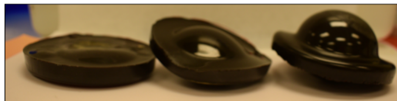
L-DOPA solution absorbed by beads & placed in Sylgard/Epoxy
