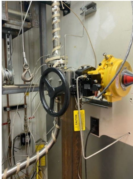
FIGURE 1. Prototype Valve Mounted in Piping
