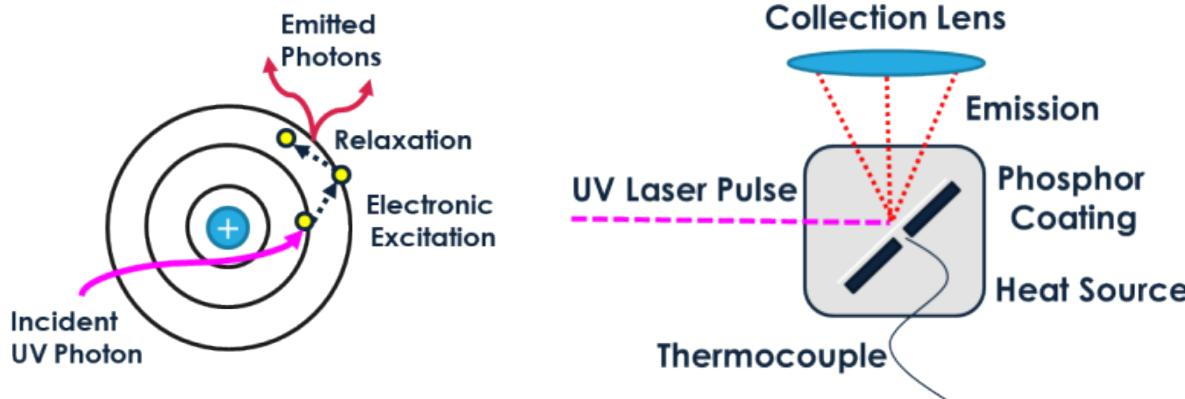
The spectral emission is temperature dependent
