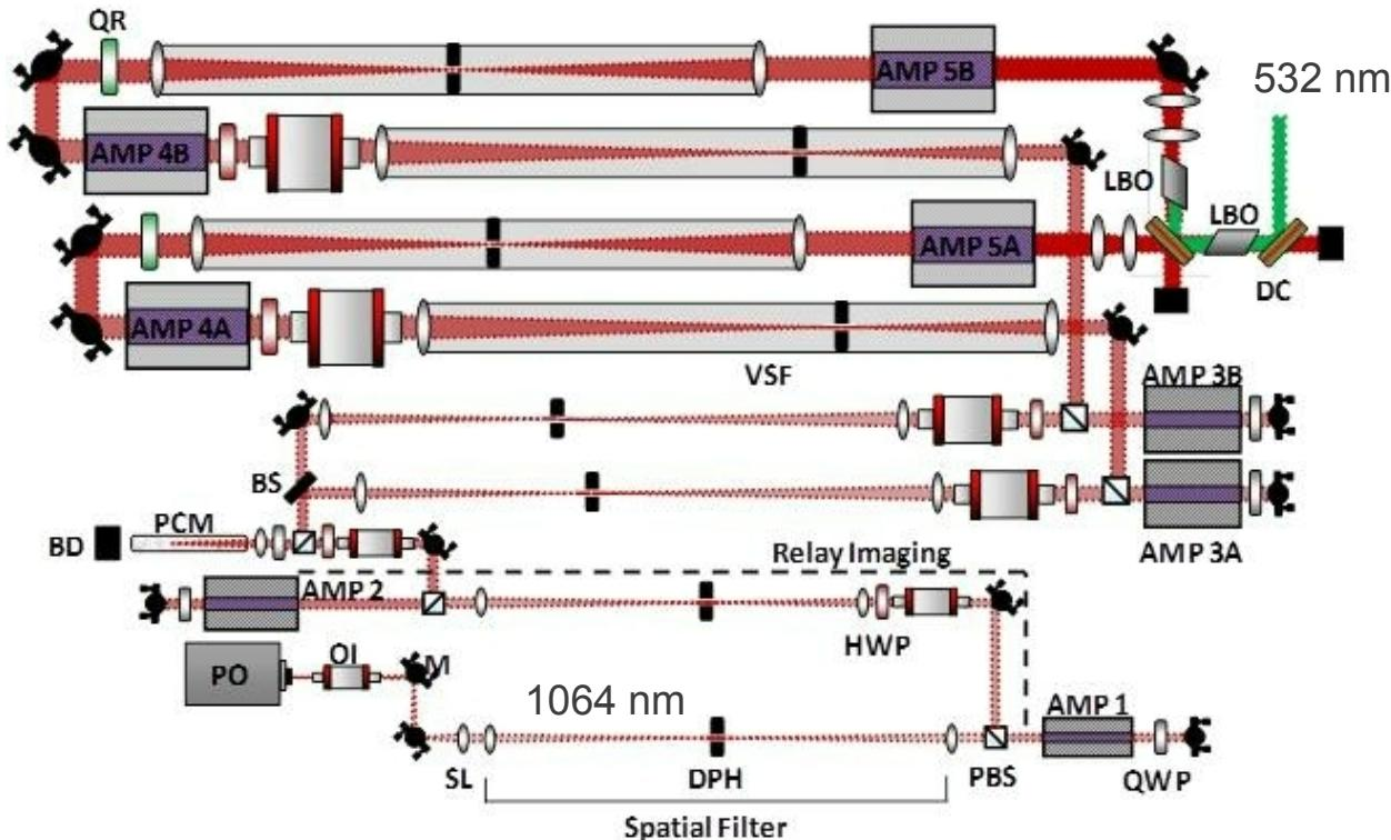
**Output is > 2.0 J/pulse per leg at 1064 nm at 10 kHz**
