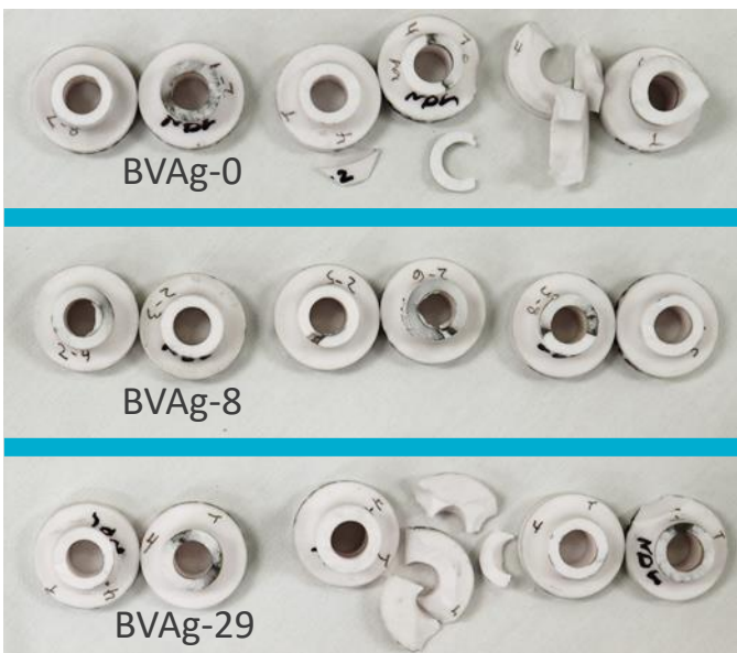
Fractured ASTM F-19 Tensile Buttons.
