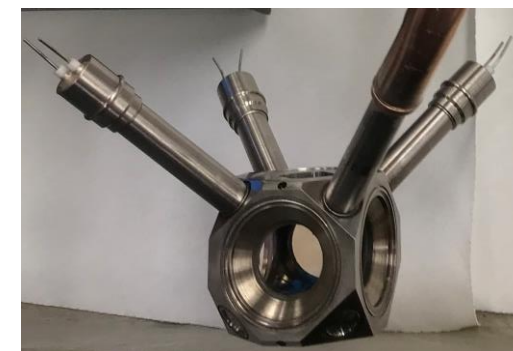
Completed titanium vacuum package
