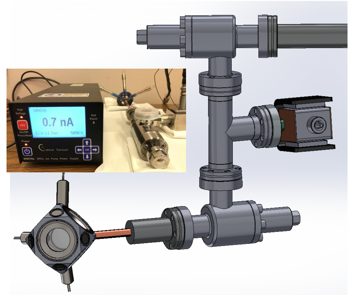
Solid-model of Titanium chamber/UHV manifold assembly
