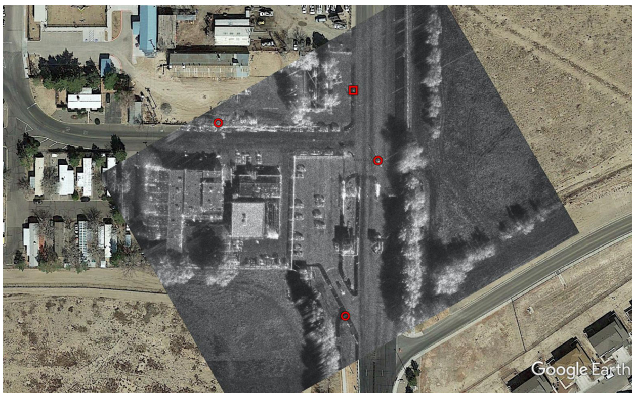
Figure 8. SAR image manually aligned to tie points. Feature to geolocate is fire hydrant marked by red box.
