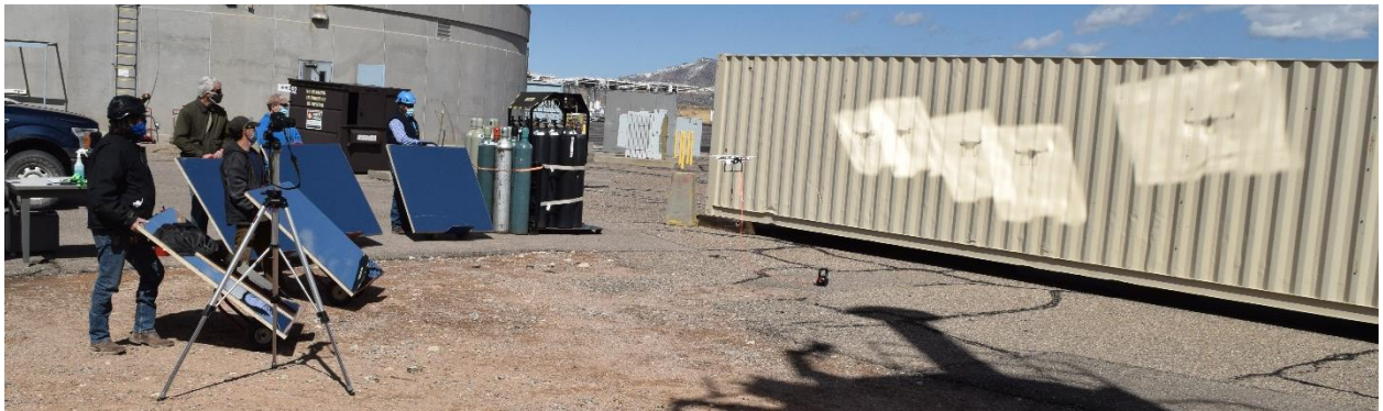
FIGURE 8. Flight test with six suns irradiance (5 mirrors plus 1 overhead).
